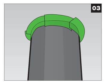
• Apply Rissan around circular parts in layers
